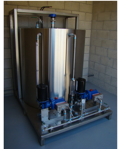
Chemical Storage and Metering Systems
